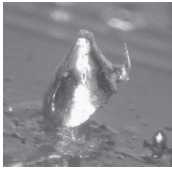
Figure 6 – Example of defect found: open joint.
