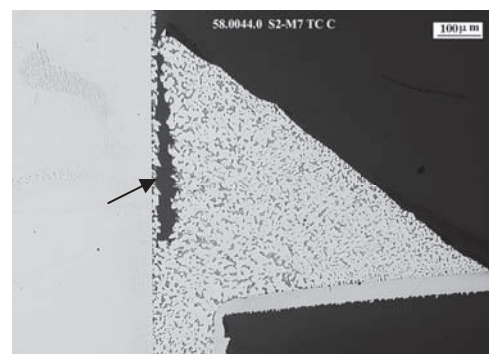
Figure 11 – Optical micrograph of sample from board E: 63Sn/37Pb; thermal cycling (3000 cycles; 0°C to 100°C) (100X). Intergranular crack propagation near the lead (arrow).
