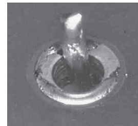
Figure 5 – Example of poor wetting defect. [16]
